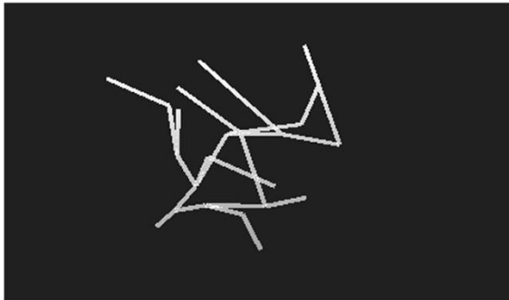
Example of current roadmap generation using an L-System approach
